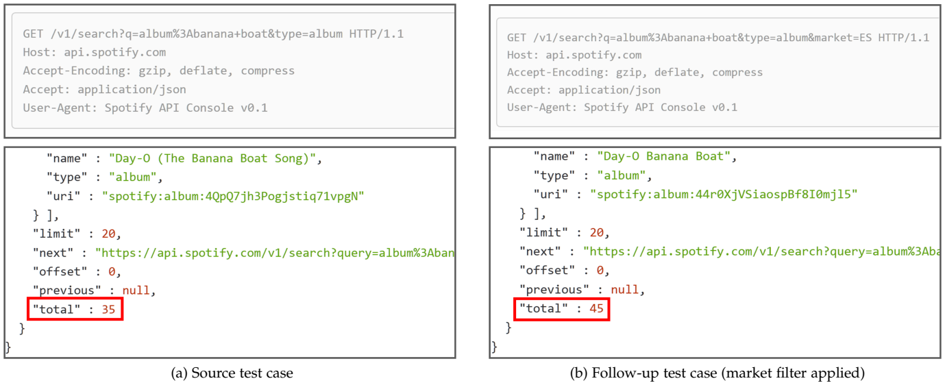
Figure 5: Metamorphic test revealing a bug in Spotify
