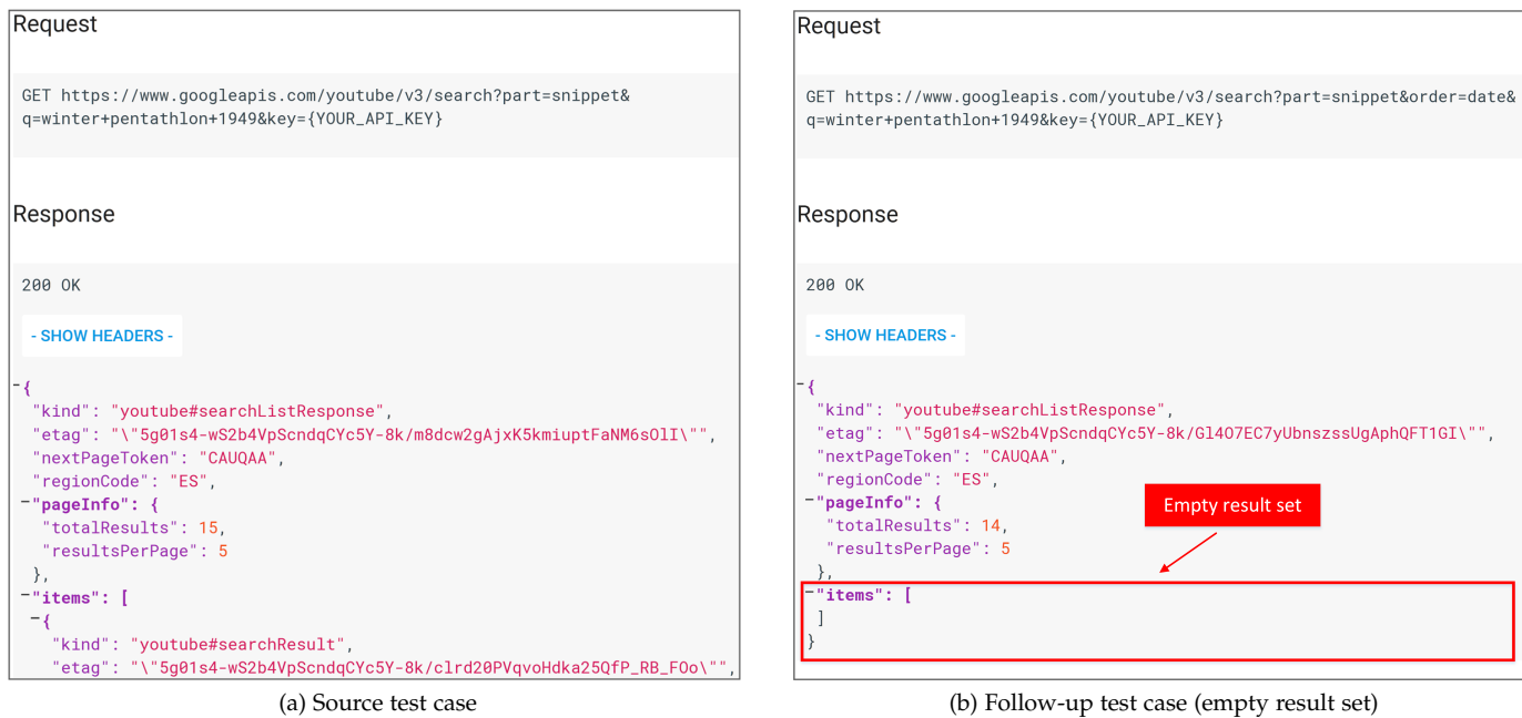
Figure 4: Metamorphic test revealing a bug in Youtube
