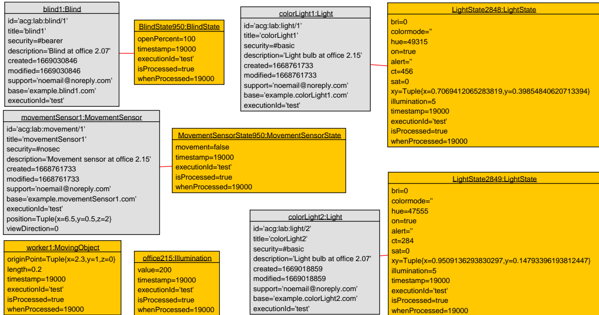
Figure 6: Excerpt of the final state of the system with one person, one blind, one motion sensor and two of the lights, plus the state of the luminosity of one of the offices.
